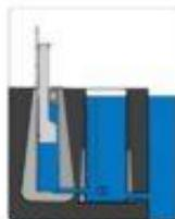
When floodwater rises to within 10cm below flood level, the enclosed basin, which houses the floating wall, starts to fill up through an inlet pipe from the adjacent service pit. The flood wall floats and rises.
